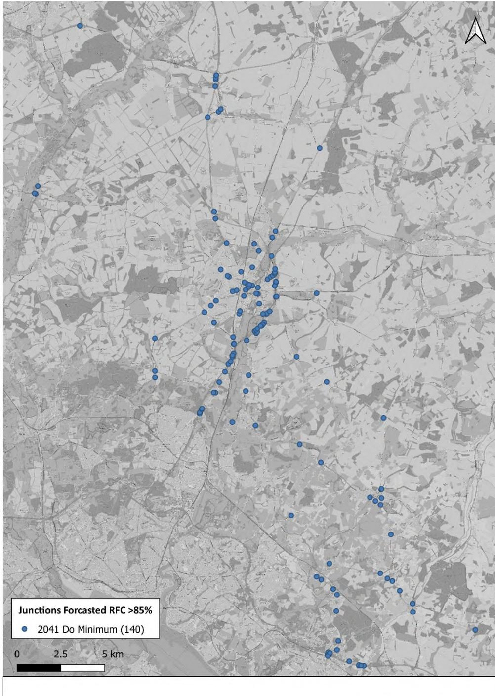
**Figure 6-10 Junctions with V/C > 85 % in 2041 Do Minimum**
