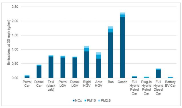
Figure 7-8 - National Average Fleet Mix (2020) - Emission Rates for the Main Vehicle Types at 30mph
