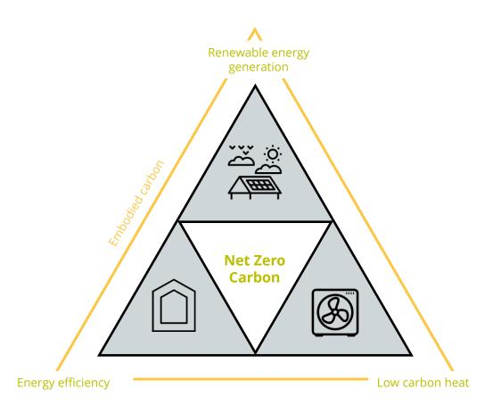
The four core principles of a "Net Zero" building: energy efficiency, low carbon heat, renewable energy generation and embodied carbon.
